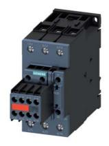
power contactor, AC-3e/AC-3, 51 A, 22 kW / 400 V, 3-pole, 110 V AC, 50 Hz / 120 V, 60 Hz, auxiliary contacts: 2 NO + 2 NC, screw terminal, size: S2, captive auxiliary switch
