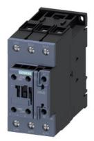
power contactor, AC-3e/AC-3, 65 A, 30 kW / 400 V, 3-pole, 20-33 V AC/DC, 50/60 Hz, with integrated varistor, auxiliary contacts: 1 NO + 1 NC, screw terminal, size: S2
