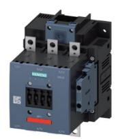
power contactor, AC-3e/AC-3 150 A, 75 kW / 400 V AC (50-60 Hz) / DC Uc: 110-127 V 3-pole, auxiliary contacts 2 NO + 2 NC permanently mounted drive: conventional main circuit: busbar control and auxiliary circuit: screw terminal
