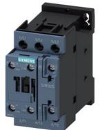
power contactor, AC-3e/AC-3, 38 A, 18.5 kW / 400 V, 3-pole, 220 V AC, 50/60 Hz, auxiliary contacts: 1 NO + 1 NC, screw terminal, size: S0
