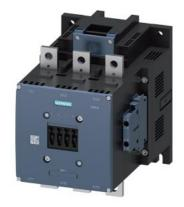
power contactor AC-1 690 A / 690 V / 40  $^{\circ}$ C 3-pole, Uc: 110-127 V AC(50-60 Hz) / DC drive: conventional auxiliary contacts 2 NO + 2 NC main circuit: busbar control and auxiliary circuit: screw terminal
