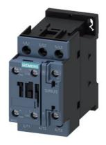
power contactor, AC-3e/AC-3, 38 A, 18.5 kW / 400 V, 3-pole, 220 V AC, 50 Hz / 240 V, 60 Hz, auxiliary contacts: 1 NO + 1 NC, screw terminal, size: S0
