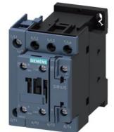
contactor AC-1, 35 A, 400 V / 40 °C, 4-pole, 110 V AC, 50 Hz / 120 V, 60 Hz, auxiliary contacts: 1 NO + 1 NC, screw terminal, size: S0
