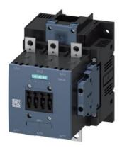
power contactor AC-1 275 A / 690 V / 40  $^{\circ}$ C 3-pole, Uc: 110-127 V AC(50-60 Hz) / DC drive: conventional auxiliary contacts 2 NO + 2 NC main circuit: busbar control and auxiliary circuit: screw terminal
