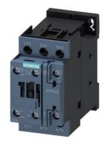
power contactor, AC-3e/AC-3, 12 A, 5.5 kW / 400 V, 3-pole, 220 V AC, 50 Hz / 240 V, 60 Hz, auxiliary contacts: 1 NO + 1 NC, screw terminal, size: S0
