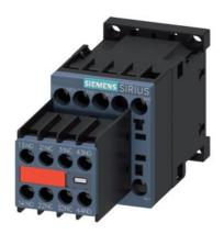
power contactor, AC-3e/AC-3, 9 A, 4 kW / 400 V, 3-pole, 24 V DC, with integrated diode, auxiliary contacts: 2 NO + 2 NC, screw terminal, size: S00, captive auxiliary switch
