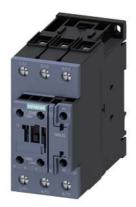
power contactor, AC-3e/AC-3, 41 A, 18.5 kW / 400 V, 3-pole, 110 V AC, 50 Hz / 120 V, 60 Hz, auxiliary contacts: 1 NO + 1 NC, screw terminal, size: S2
