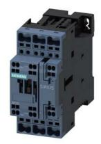
power contactor, AC-3e/AC-3, 38 A, 18.5 kW / 400 V, 3-pole, 24 V DC, auxiliary contacts: 1 NO + 1 NC, spring-loaded terminal, size: S0  $\,$
