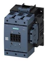
power contactor, AC-3e/AC-3 115 A, 55 kW / 400 V, AC (50-60 Hz) / DC Uc: 110-127 V 3-pole, auxiliary contacts 2 NO + 2 NC drive: conventional main circuit: box terminal control and auxiliary circuit: screw terminal
