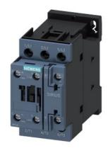
power contactor, AC-3e/AC-3, 12 A, 5.5 kW / 400 V, 3-pole, 110 V AC, 50 Hz / 120 V, 60 Hz, auxiliary contacts: 1 NO + 1 NC, screw terminal, size: S0
