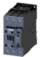
power contactor, AC-3e/AC-3, 41 A, 18.5 kW / 400 V, 3-pole, 24 V DC, 0.8-1.2\* Us, with integrated varistor, auxiliary contacts: 1 NO + 1 NC, screw terminal, size: S2, suitable for PLC outputs
