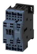
power contactor, AC-3e/AC-3, 38 A, 18.5 kW / 400 V, 3-pole, 110 V AC, 50 Hz / 120 V, 60 Hz, auxiliary contacts: 1 NO + 1 NC, spring-loaded terminal, size: S0
