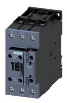
power contactor, AC-3e/AC-3, 65 A, 30 kW / 400 V, 3-pole, 24 V DC, 0.8-1.2\* Us, with integrated varistor, auxiliary contacts: 1 NO + 1 NC, screw terminal, size: S2, suitable for PLC outputs
