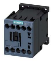
power contactor, AC-3e/AC-3, 16 A, 7.5 kW / 400 V, 3-pole, 220 V AC, 50 Hz / 240 V, 60 Hz, auxiliary contacts: 1 NO, screw terminal, size: S00
