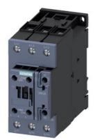
power contactor, AC-3e/AC-3, 51 A, 22 kW / 400 V, 3-pole, 24 V DC, 0.8-1.2\* Us, with integrated varistor, auxiliary contacts: 1 NO + 1 NC, screw terminal, size: S2, suitable for PLC outputs
