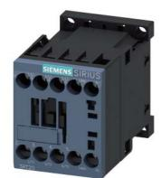
power contactor, AC-3e/AC-3, 12 A, 5.5 kW / 400 V, 3-pole, 110 V AC, 50 Hz / 120 V, 60 Hz, auxiliary contacts: 1 NO, screw terminal, size: S00
