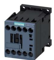
power contactor, AC-3e/AC-3, 16 A, 7.5 kW / 400 V, 3-pole, 24 V DC, auxiliary contacts: 1 NO, screw terminal, size: S00  $\,$
