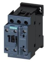
power contactor, AC-3e/AC-3, 17 A, 7.5 kW / 400 V, 3-pole, 110 V AC, 50 Hz / 120 V, 60 Hz, auxiliary contacts: 1 NO + 1 NC, screw terminal, size: S0
