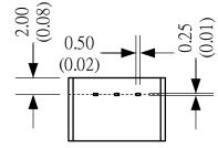
Dimensions are in mm (inch) Pin Tolerance :  $\pm 0.05$  mm (0.002 inch) Pin Distance :  $\pm 0.25$  mm (0.01 inch) Case Tolerance :  $\pm 0.50$  mm (0.02 inch)
